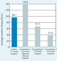
Benchtop engineering test utilizing a dense bone substrate.
