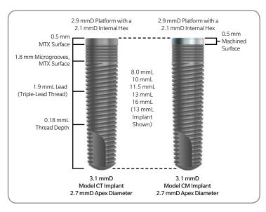
The 3.1 mmD Eztetic Dental Implants have a MTX microtextured or 0.5 mm machined coronal aspect, followed by 1.8 mm of the MTX Surface with microgrooves. The six microgrooves are circumferential with a depth of 0.06 mm and peak-to-peak width of 0.3 mm. Triple-lead threads begin immediately after the microgrooves and continue to the apex. The degree of body taper varies between 1° and 4°, depending on implant length.
